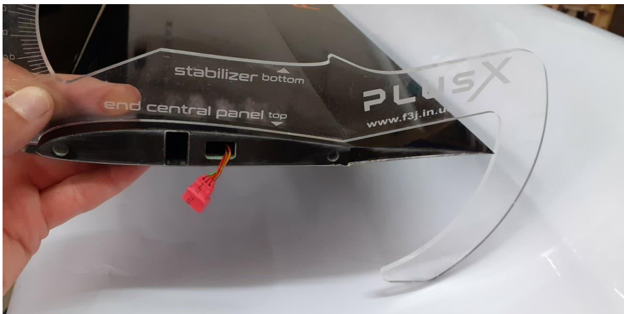
Tool to accurately measure the travel of surfaces to symmetry the settings for example.
