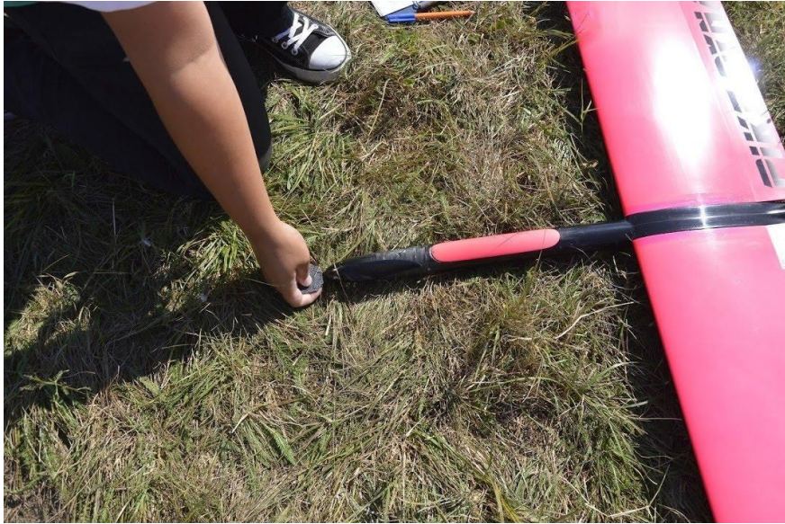
Checking the cone with a template when registering models at CDE 2018
